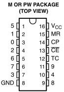
and sequentially goes high on the low-to-high transition clock period of the ten-clock-period cycle. The carry (TC) output transitions low to high after output 9 goes from high to low, and can be used in conjunction with the clock enable (CE) input to cascade several stages. CE disables counting when in the high state. A master reset (MR) input also is provided that, when taken high, sets all the decoded outputs, except output 0, to low.
