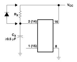
Figure 5. Rapid-Power-Down Protection Circuit
