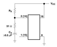
Figure 6. Alternative Rapid-Power-Down Protection Circuit
