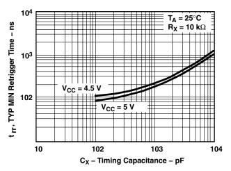
Figure 4. Minimum Retrigger Time vs Timing Capacitance
