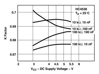
Figure 2. K Factor vs DC Supply Voltage
