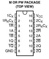
external capacitor  $(C_X)$  control the timing and accuracy for the circuit. Adjustment of  $R_X$  and  $C_X$  provides a wide range of output pulse widths from the Q and  $\overline{Q}$  terminals. The propagation delay from trigger input-to-output transition and the propagation delay from reset input-to-output transition are independent of  $R_X$  and  $C_X$ .
