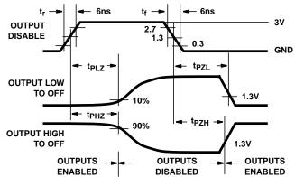
FIGURE 8. HC THREE-STATE PROPAGATION DELAY WAVEFORM
