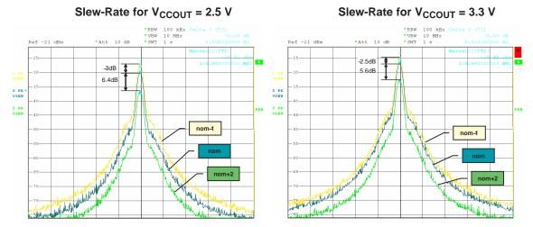
Figure 22. EMI Reduction vs Slew-Rate and V<sub>ccout</sub>
