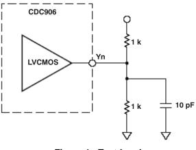
Figure 1. Test Load
