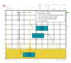
Figure 31. Noise Coupling and Spur Suppression
