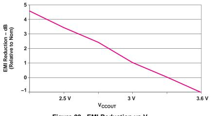
Figure 23. EMI Reduction vs V<sub>ccout</sub>
