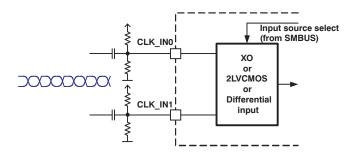
Figure 18. Differential Clock Input Circuitry
