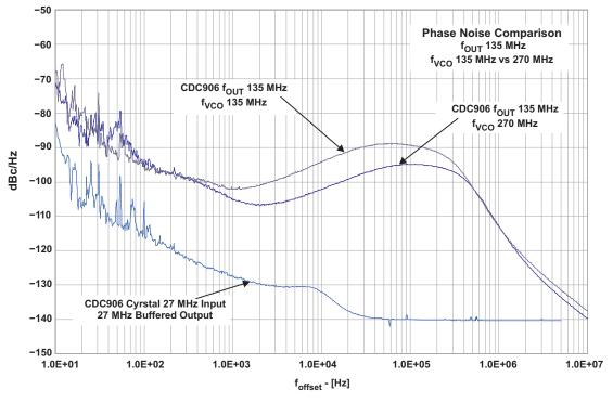
Figure 33. Phase Noise Characteristic
