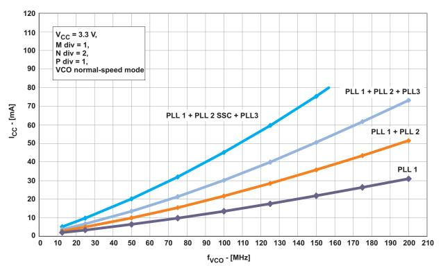
Figure 2. I<sub>CC</sub> vs Number of PLLs and VCO Frequency (VCO at Normal-Speed Mode, Byte 6 Bit [7:5])
