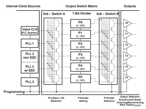
Figure 24. CDC906 Output Switch Matrix
