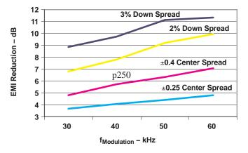
Figure 21. EMI Reduction vs f<sub>Modulation</sub> and f<sub>Amount</sub>
