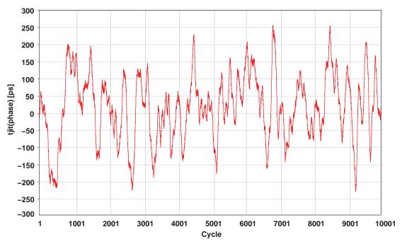
Figure 29. Snapshot of Phase Jitter
