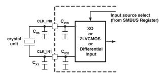
Figure 15. Crystal Input Circuitry
