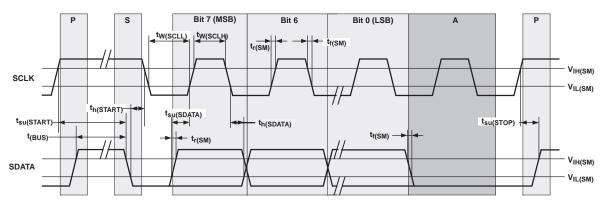
Figure 11. Timing Diagram Serial Control Interface
