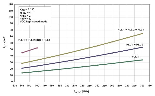
Figure 3. I<sub>CC</sub> vs Number of PLLs and VCO Frequency (VCO at High-Speed Mode, Byte 6 Bit [7:5])
