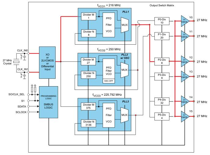
NOTE: All outputs are enabled and in non-inverting mode. S0, S1, and SSC comply according the default setting described in Byte 10 and Byte 25 respectively.
