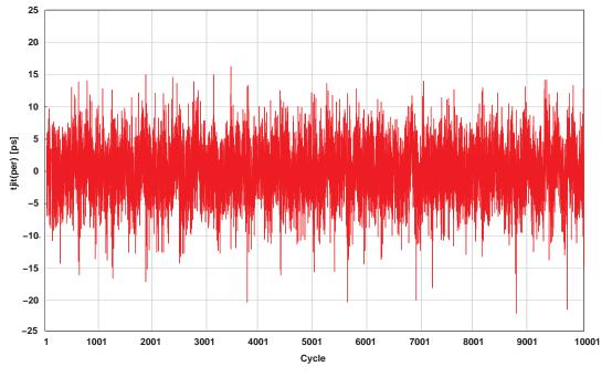
Figure 28. Snapshot of Period Jitter
