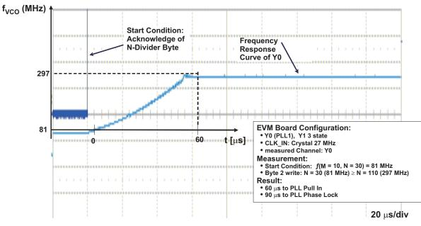
Figure 34. Snapshot of the PLL Lock-Time
