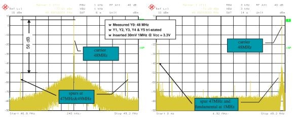
Figure 32. Power Supply Noise Rejection
