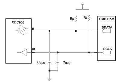
Figure 12. SMBus Hardware Interface
