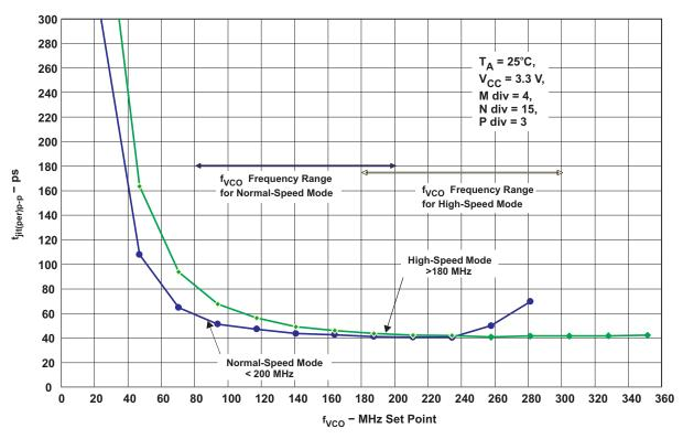
Figure 30. Period Jitter vs f<sub>VCO</sub> for Normal-Speed Mode and High-Speed Mode
