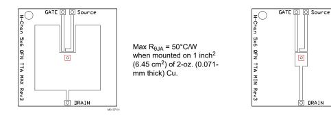
Max  $R_{\theta JA}$  = 123°C/W when mounted on minimum pad area of 2-oz. (0.071-mm thick) Cu.
