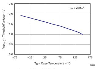
Figure 6. Threshold Voltage vs. Temperature
