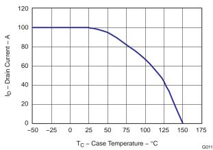
Figure 12. Maximum Drain Current vs. Temperature
