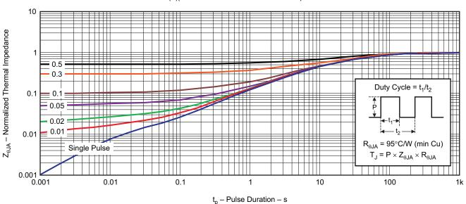
Figure 1. Transient Thermal Impedance
