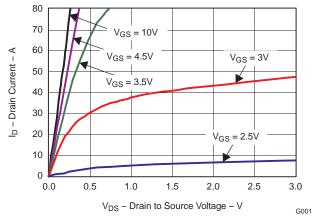
Figure 2. Saturation Characteristics
