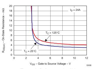
Figure 7. On Resistance vs. Gate Voltage
