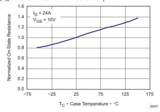
Figure 8. On Resistance vs. Temperature
