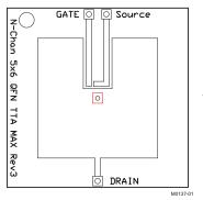
Max  $R_{\theta JA} = 51$ °C/W when mounted on 1 inch<sup>2</sup> of 2 oz. Cu.
