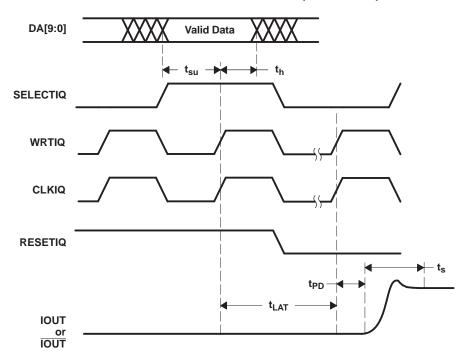
Figure 17. Single-Bus Interleaved-Mode Operation
