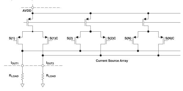
Figure 18. Analog Outputs
