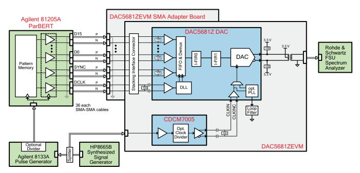
Figure 34. DAC5681Z Test Configuration for Normal Clock Mode
