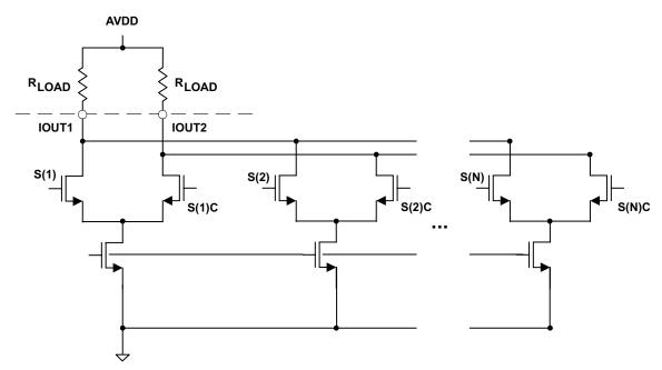
Figure 36. Equivalent Analog Current Output
