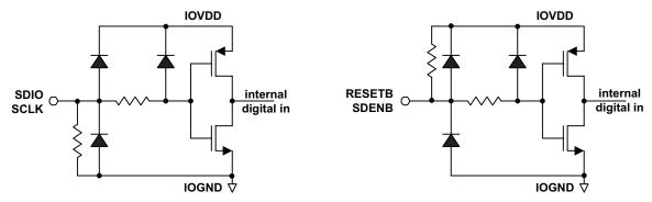
Figure 35. CMOS/TTL Digital Equivalent Input
