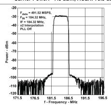
Figure 15. Single Carrier W-CDMA Test Model 1 Carrier Power: –8.9 dBm, ACLR: 72 dB
