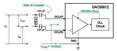
Figure 32. LVDS Clock (DCLKP/N) Input Levels
