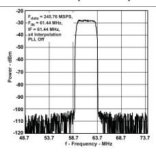
Figure 13. Single Carrier W-CDMA Test Model 1 Carrier Power: -7.8 dBm, ACLR: 79.3 dB
