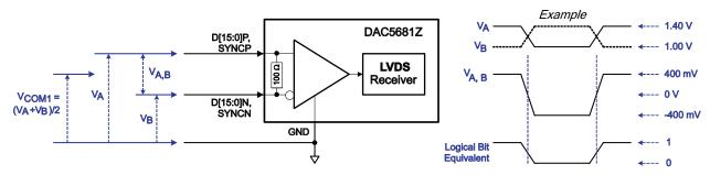
Figure 31. LVDS Data (D[15:0]P/N, SYNCP/N Pairs) Input Levels
