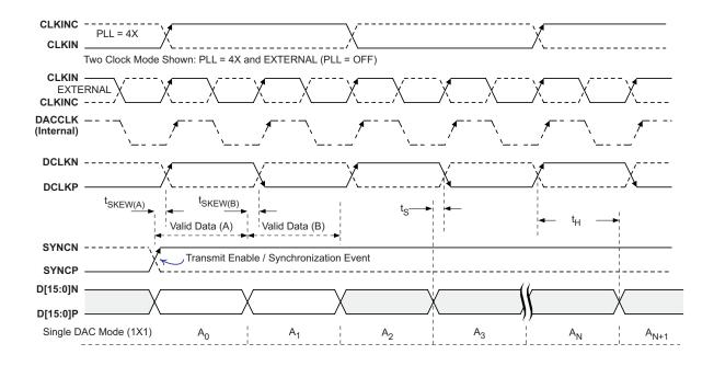
Figure 42. Clock and Data Timing Diagram
