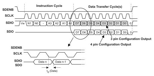
Figure 48. Serial Interface Read Timing Diagram
