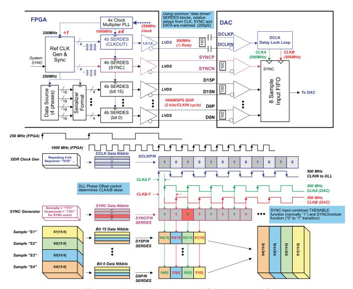
Figure 29. Example FPGA-Based LVDS Data Flow to DAC
