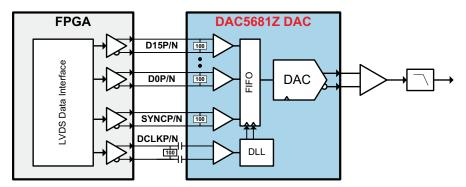
Figure 41. System Diagram of Arbitrary Waveform Generator
