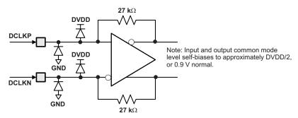
Figure 44. DCLKP/N Equivalent Input Circuit
