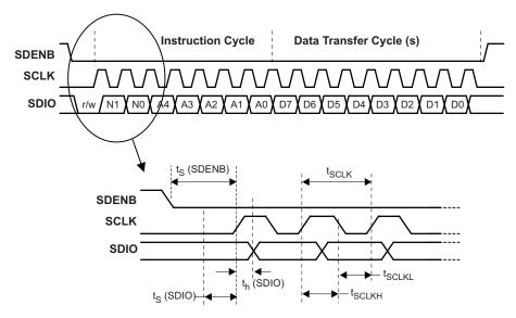
Figure 47. Serial Interface Write Timing Diagram
