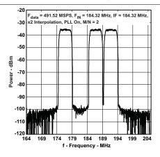
Figure 24. Three Carrier W-CDMA Test Model 1 With Gap Carrier Power: -15.7 dBm, ACLR: 65.9 dB
