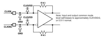
Figure 45. CLKIN/C Equivalent Input Circuit
