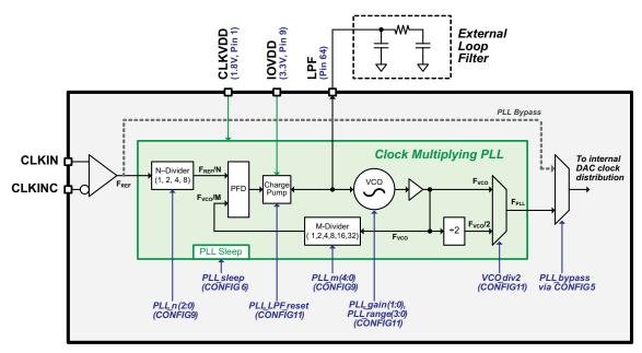
Figure 43. Functional Block Diagram for PLL
