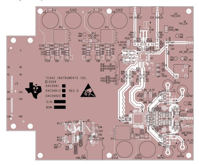
Figure 67. Top Layer of DAC5681Z EVM Layout
