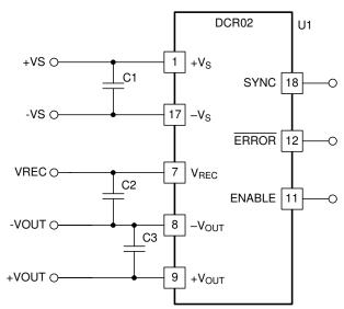
Figure 10-3. DCR02 PCB Schematic, U Package
