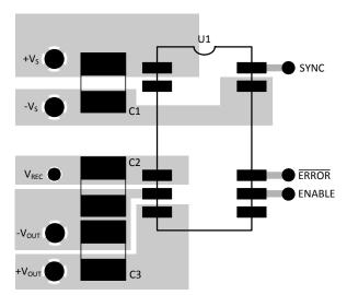
Figure 10-1. PCB Layout Example, Component-Side View
