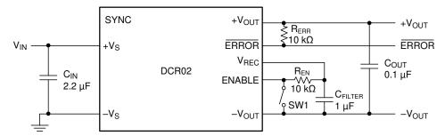
Low-ESR, ceramic capacitors are required for  $C_{\text{IN}}$ ,  $C_{\text{OUT}}$ , and  $C_{\text{FILTER}}$ .
