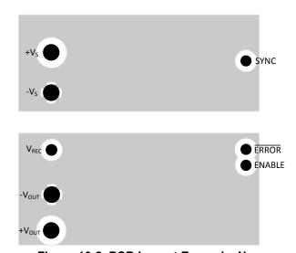
Figure 10-2. PCB Layout Example, Non-Component-Side View
