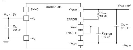
Low-ESR, ceramic capacitors are required for  $C_{\text{IN}}$ ,  $C_{\text{OUT}}$ , and  $C_{\text{FILTER}}$ .
