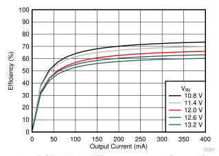
Figure 8-5. DCR021205 Efficiency versus Output Current
