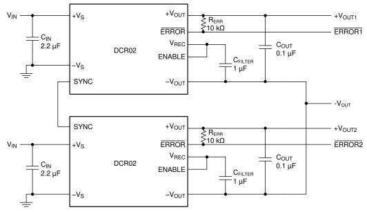
Low-ESR, ceramic capacitors are required for CIN, COUT, and CFILTER.
