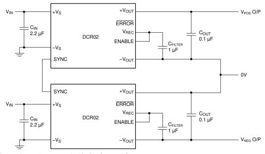
Low-ESR, ceramic capacitors are required for  $C_{\text{IN}}$ ,  $C_{\text{OUT}}$ , and  $C_{\text{FILTER}}$ .
