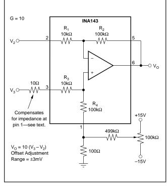
FIGURE 3. Offset Adjustment.
