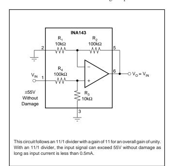
FIGURE 6. Voltage Follower with Input Protection.
