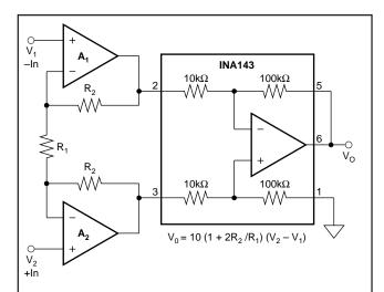
The INA143 can be combined with op amps to form a complete instrumentation amplifier with specialized performance characteristics. Burr-Brown offers many complete high performance IAs. Products with related performances are shown at the right in the table below.
