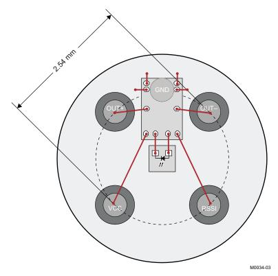
Figure 18. TO46 5-Pin Layout Example Using the ONET4291T
