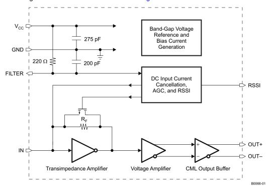
Figure 1. Simplified Block Diagram of the ONET4291T
