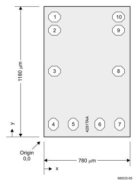
Figure 16. Chip Dimensions and Pad Locations
