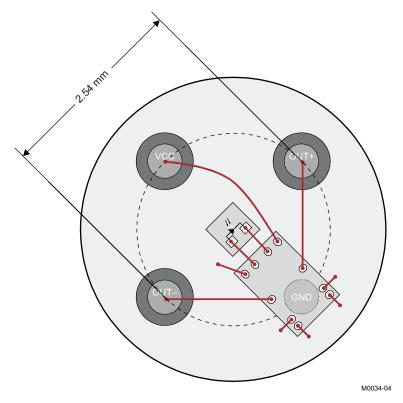
Figure 19. TO46 4-Pin Layout Example Using the ONET4291T
