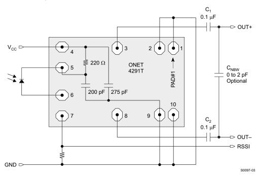
Figure 15. Basic Application Circuit
