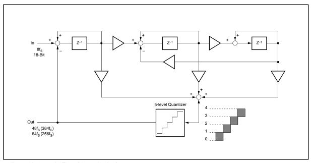
FIGURE 10. 5-Level  $\Delta\Sigma$  Modulator Block Diagram.
