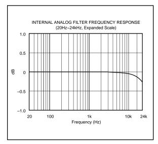
FIGURE 7. Low Pass Filter Frequency Response.
