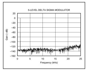
FIGURE 11. Quantization Noise Spectrum.
