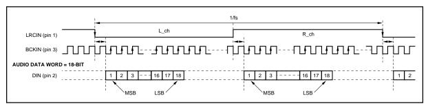
FIGURE 2. "I2S" Data Input Timing.
