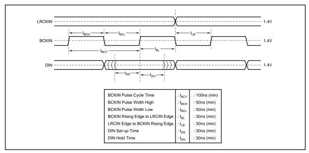
FIGURE 3. Audio Data Input Timing.
