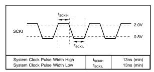
FIGURE 4. System Clock Timing Requirements.
