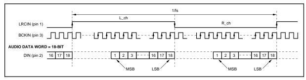
FIGURE 1. "Normal" Data Input Timing.
