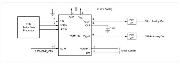
FIGURE 5. Typical Connection Diagram.
