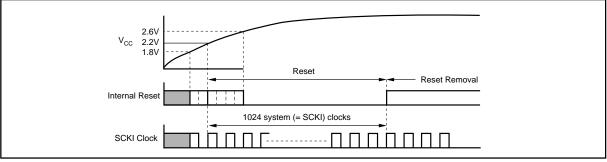
FIGURE 6. Internal Power-On Reset Timing.
