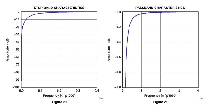
**TYPICAL CHARACTERISTICS: ADC ANALOG ANTIALIASING FILTER FREQUENCY RESPONSE** All specifications at  $T_A = +25^{\circ}$ C,  $V_{BUS} = 5$  V,  $f_S = 44.1$  kHz,  $f_{in} = 1$  kHz, 16-bit data, unless otherwise noted.
