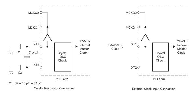
Figure 8. Master Clock Generator Connection Diagram
