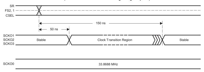
Figure 10. SCKO Transient Timing
