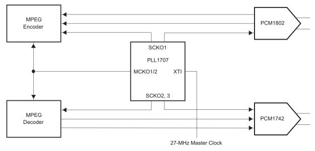
Figure 14. Block Diagram of HDD+DVD Recorder Application
