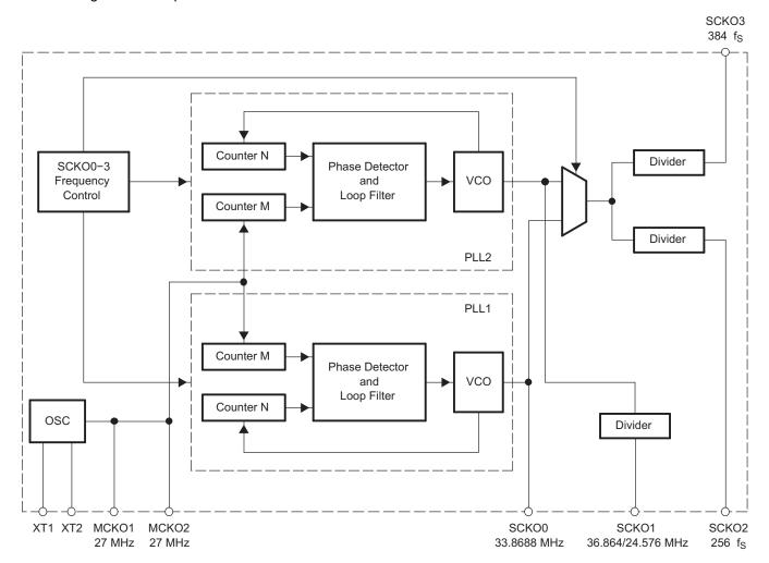
Figure 7. Block Diagram
