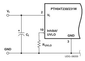
Figure 18. Undervoltage Lockout
