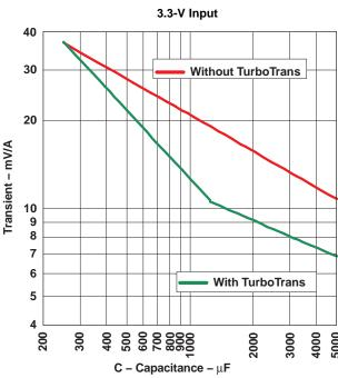
Figure 13. Capacitor Type B,  $1000 < C(\mu F) \times ESR(m\Omega) \le$ (e.g. Polymer-Tantalum)
