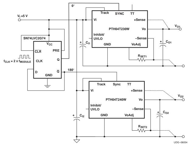
Figure 23. Typical SmartSync Circuit
