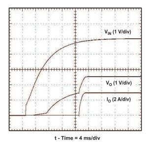
Figure 28. Prebias Startup Waveforms
