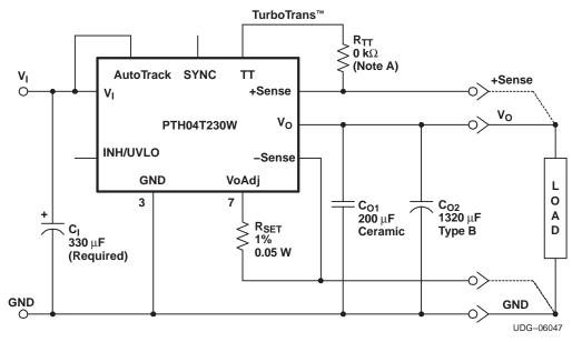
A. The value of  $R_{TT}$  must be calculated using the total value of output capacitance.
