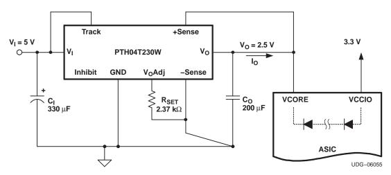
Figure 27. Application Circuit Demonstrating Prebias Startup
