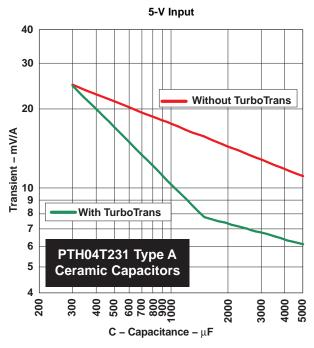
3.3-V Input 40 30 Without TurboTrans 20 Transient – mV/A 10 8 With TurboTrans 7 6 PTH04T231 Type A 5 **Ceramic Capacitors** 400 500 600 700 800 900 900 200 C - Capacitance - μF
