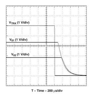
Figure 26. Simultaneous Power Down With Auto-Track
