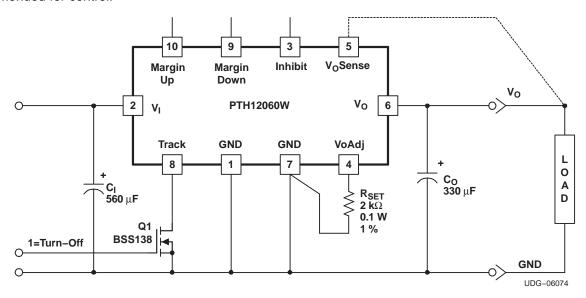
Figure 12. Basic Start-up Control Circuit
