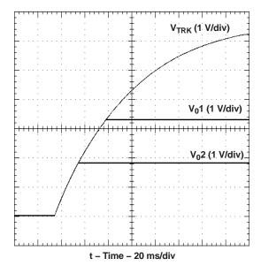
Figure 15. Simultaneous Power Up With Auto-Track Control
