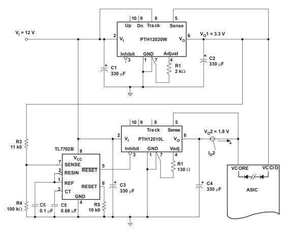
Figure 18. Application Circuit Demonstrating Prebias Startup
