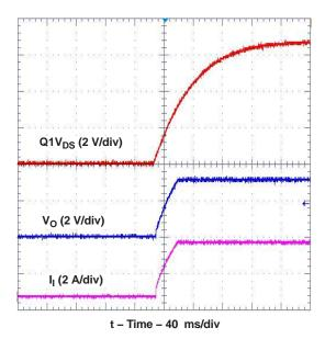
Figure 13. Power-Up from Track Control
