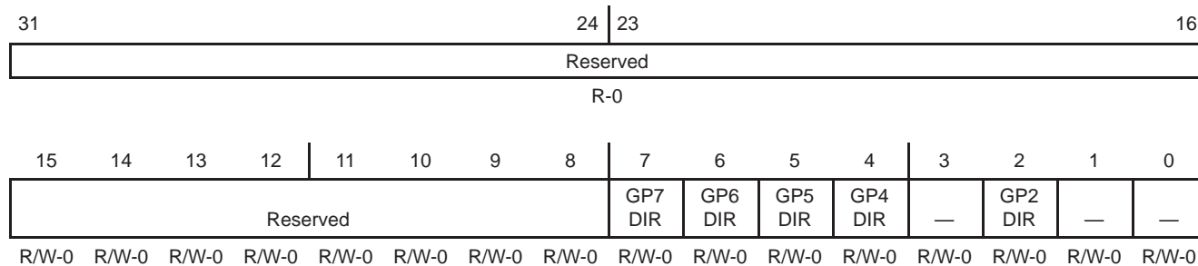
Figure 12. GPIO Direction Register (GPDIR) [Hex Address: 01B0 0004]
