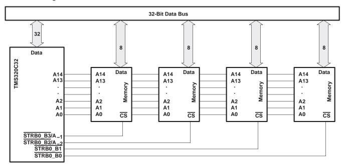
Figure 4. 'C32 With 32-Bit-Wide External Memory
