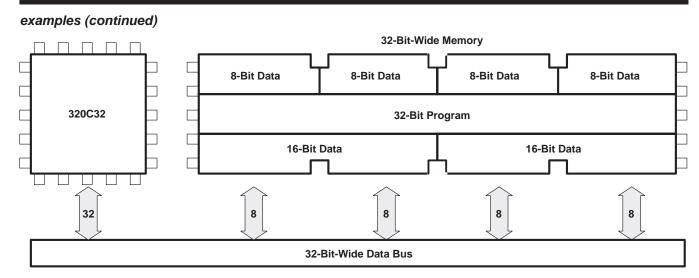
Figure 5. 'C32 With 32-Bit-Wide External Memory Configured With 8- and 16-Bit Data Areas and 32-Bit Program Memory
