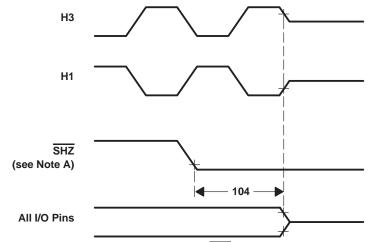
NOTE A: Enabling SHZ destroys 'C32 register and memory contents. Assert SHZ = 1 and reset the 'C32 to restore it to a known condition.
