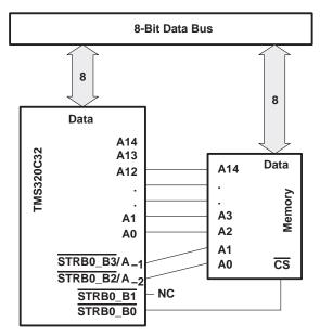
Figure 2. 'C32 With 8-Bit-Wide External Memory
