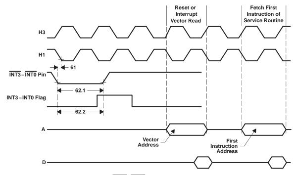
Figure 27. INT3-INT0 Interrupt-Response Timing
