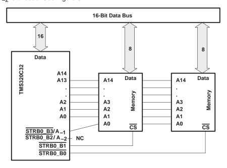
Figure 3. 'C32 With 16-Bit-Wide External Memory
