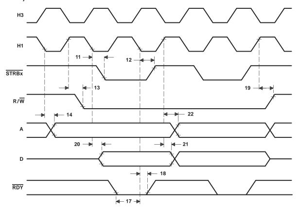
Figure 17. Memory-Write-Cycle Timing
