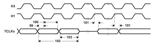
Figure 35. Timing for Timer Pin
