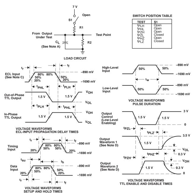
NOTES: A.C<sub>I</sub> includes probe and jig capacitance.
