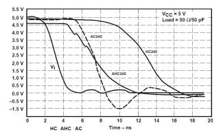
Figure 8-2. Switching Characteristics Comparison
