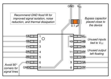
Figure 9-1. Example Layout for the SN74AHC373
