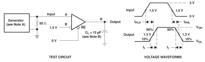
NOTES: A. The input pulse is supplied by a generator having the following characteristics: PRR  $\leq$  1 MHz, 50% duty cycle,  $t_r \leq$  6 ns,  $t_f \leq$  6 ns,  $t_f \leq$  6 ns,  $t_f \leq$  6 ns,  $t_f \leq$  1 MHz, 50% duty cycle,  $t_f \leq$  1 mHz,  $t_f \leq$  1
