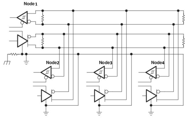
Figure 9-1. Full Duplex Application Circuit
