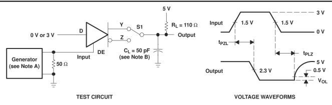
Figure 7-5. Driver Test Circuit and Enable and Disable Time Voltage Waveforms
