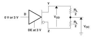
Figure 7-1. Differential and Common-Mode Output Voltages
