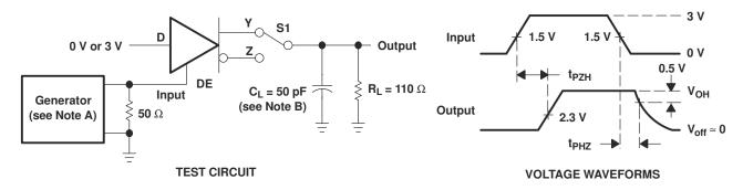
Figure 7-4. Driver Test Circuit and Enable and Disable Time Waveforms
