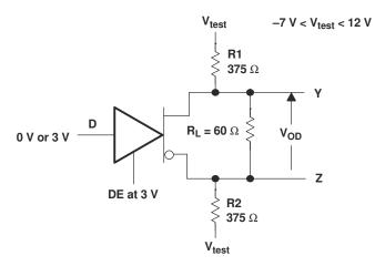
Figure 7-2. Driver V<sub>OD</sub> Test Circuit
