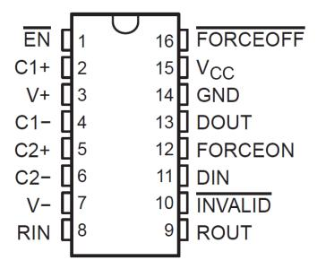
Figure 6-1. DB or PW Package Top View
