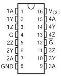
Figure 4-1. N Package (Top View)
