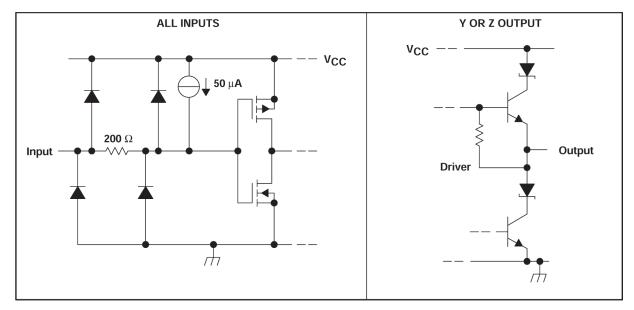
Figure 7-2. Schematic Diagrams of Inputs and Outputs
