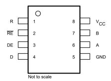
Figure 4-1. D Package, SOIC 8 Pins (Top View)
