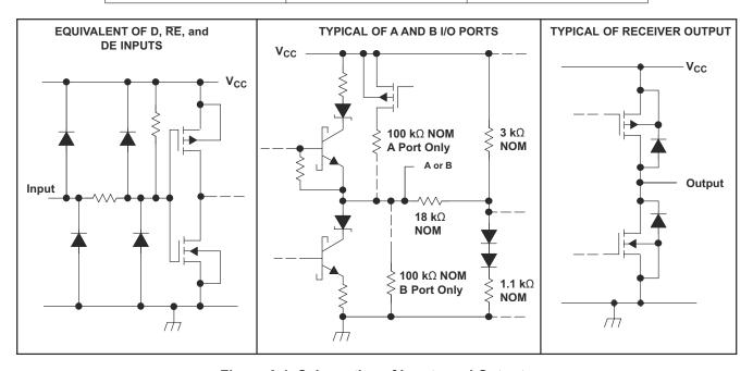
Figure 6-1. Schematics of Inputs and Outputs
