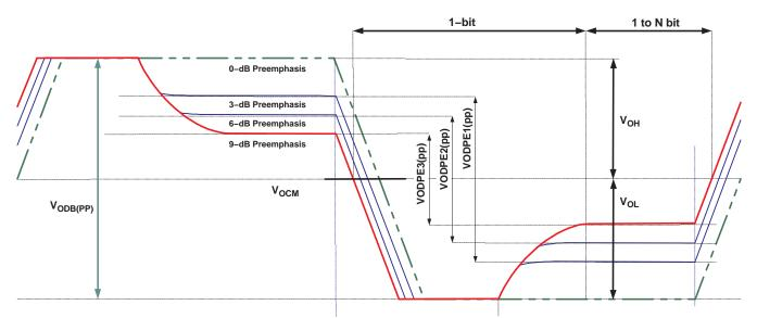
Figure 3. Preemphasis and Output Voltage Waveforms and Definitions
