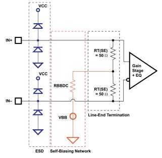
Figure 1. Equivalent Input Circuit Design
