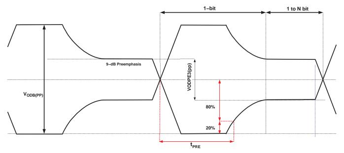
Figure 4. t<sub>(PRE</sub>) Preemphasis Duration Measurement
