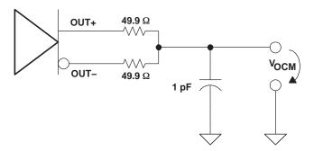
Figure 2. Common-Mode Output Voltage Test Circuit
