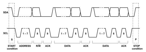
Figure 20. I<sup>2</sup>C Address and Data Cycles
