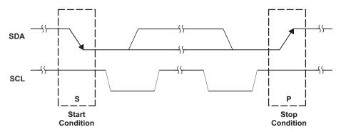
Figure 17. I<sup>2</sup>C Start and Stop Conditions
