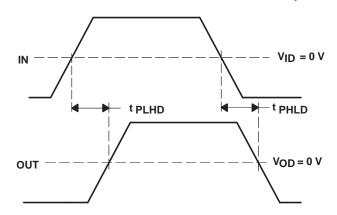
Figure 6. Propagation Delay Input to Output
