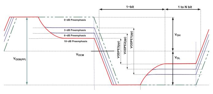
Figure 3. Preemphasis and Output Voltage Waveforms and Definitions
