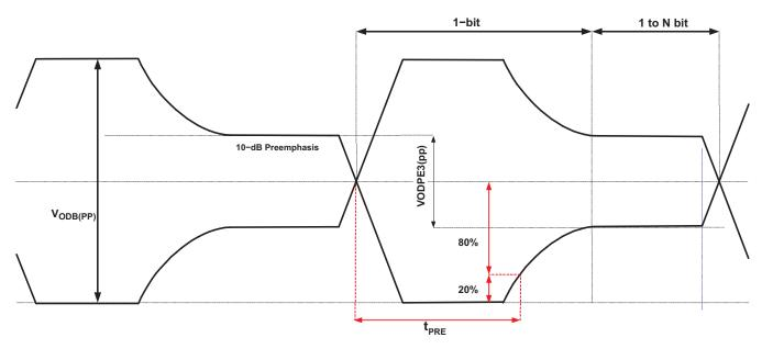
Figure 4. t<sub>(PRE)</sub> Preemphasis Duration Measurement
