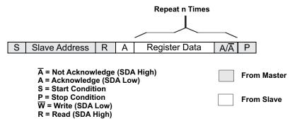
Figure 23. I<sup>2</sup>C Read Cycle
