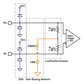
Figure 1. Equivalent Input Circuit Design
