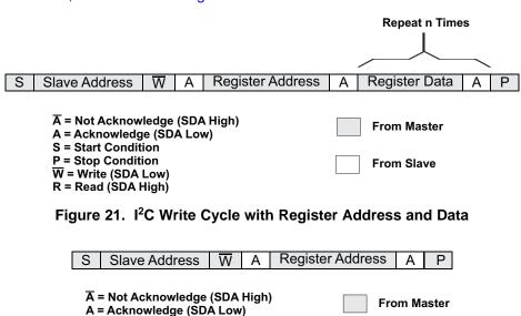
Figure 22. I<sup>2</sup>C Write Cycle with Register Address Only
