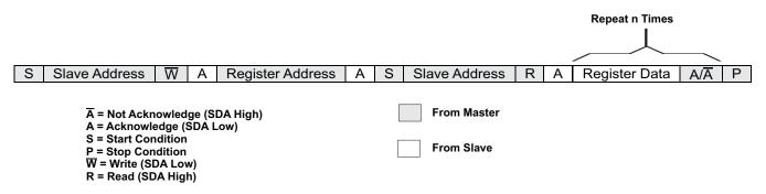
Figure 24. I<sup>2</sup>C Combined Format Write/Read Cycle
