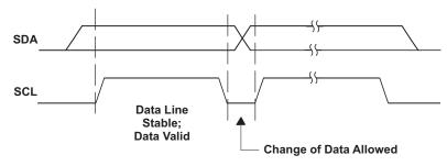
Figure 18. I<sup>2</sup>C Bit Transfer
