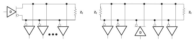
Figure 8-2. Multidrop Architectures With Different Driver Locations
