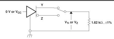
Figure 6-7. Driver Maximum Steady State Output Voltage
