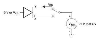
Figure 6-4. Short-Circuit Test Circuit
