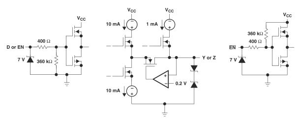
Figure 7-1. Equivalent Input and Output Schematic Diagrams
