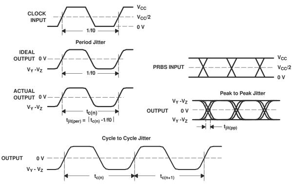
$t_{jit(cc)} = \mid t_{c(n)} - t_{c(n+1)} \mid$
