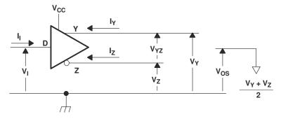
Figure 6-1. Driver Voltage and Current Definitions
