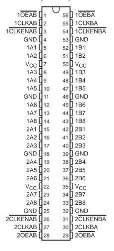
To ensure the high-impedance state during power up or power down,  $\overline{OE}$  should be tied to  $V_{CC}$  through a pullup resistor; the minimum value of the resistor is determined by the current-sinking capability of the driver.
