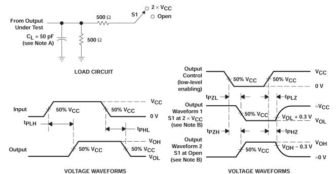
A. C<sub>L</sub> includes probe and jig capacitance.
