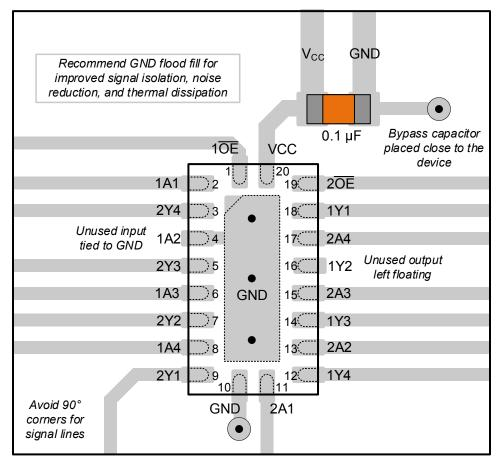
Figure 8-1. Example Layout for the SN74AC240-Q1
