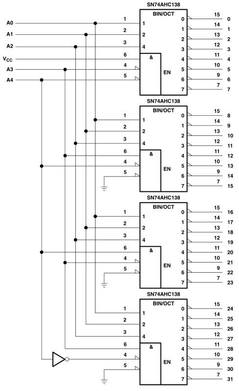
Figure 7-2. 32-Bit Decoding Scheme
