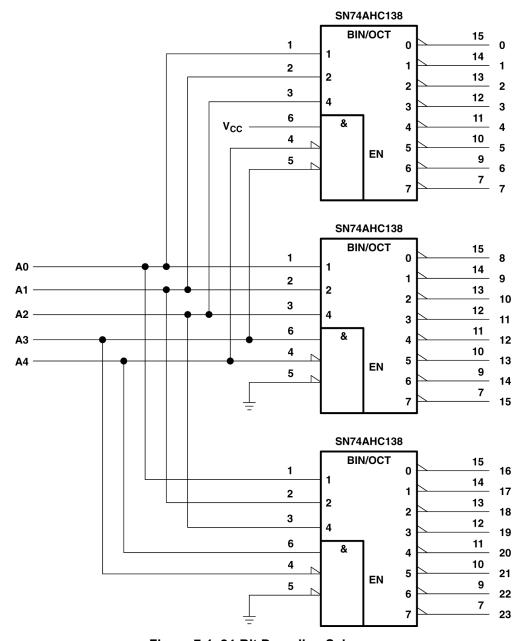
Figure 7-1. 24-Bit Decoding Scheme
