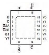
Figure 3-2. RGY Package, 16-Pin VQFN (Top View)
