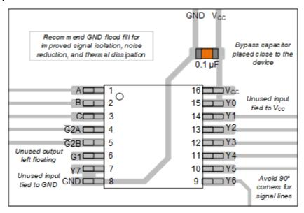
Figure 7-3. Example Layout for the SN74AHC138
