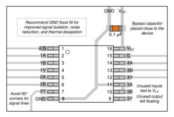
Figure 7-1. Example Layout for the SNx4AHC157
