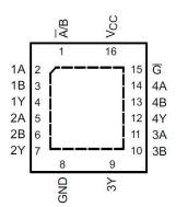
Figure 3-2. SN74AHC157 RGY Package, (Top View)
