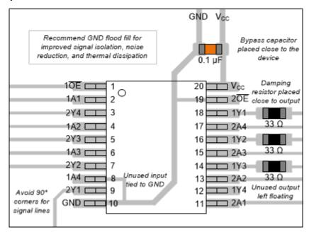
Figure 9-1. Layout Diagram
