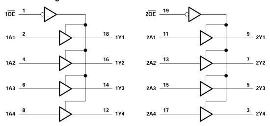
Figure 8-1. Logic Diagram (Positive Logic)
