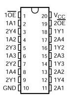
Figure 5-1. DW or PW Package (Top View)
