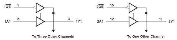
Figure 8-1. Logic Diagram (Positive Logic)
