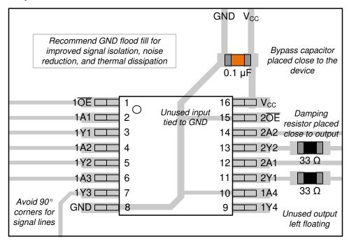
Figure 9-2. Example Layout for the SN74AHC367
