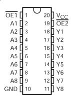
Figure 5-1. D or PW Package (Top View)
