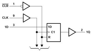
To Five Other Channels Figure 3-1. Logic Diagram (Positive Logic)
