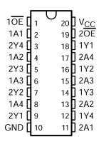
Figure 4-1. DW or PW Package (Top View)
