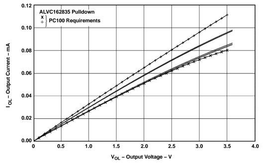
Figure 3. IV Characteristics - Pulldown
