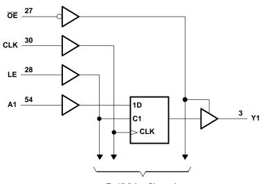
To 17 Other Channels Pin numbers shown are for the DGG, DGV, and DL packages.
