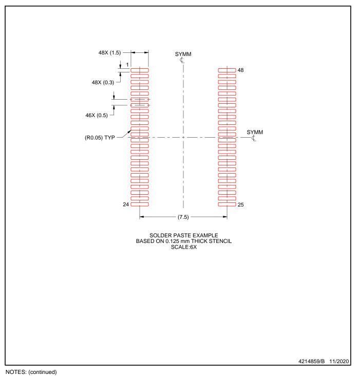
7. Laser cutting apertures with trapezoidal walls and rounded corners may offer better paste release. IPC-7525 may have alternate
