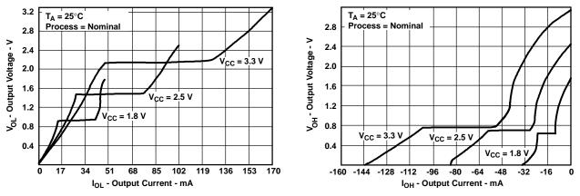
Figure 1. Output Voltage vs Output Current
