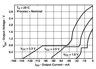
Figure 1. Output Voltage vs Output Current
