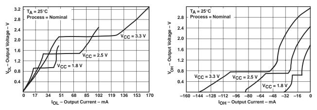
Figure 1. Output Voltage vs Output Current
