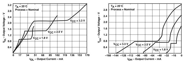
Figure 1. Output Voltage vs Output Current
