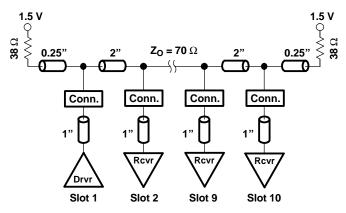
Figure 2. Medium-Drive Test Backplane
