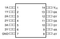
Figure 5-1. D, DGV, NS, or PW Package (Top View)
