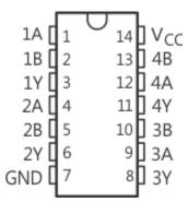
Figure 4-1. PW Package 14-Pin TSSOP Top View
