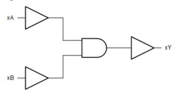
Figure 7-1. Logic Diagram, each gate (Positive Logic)
