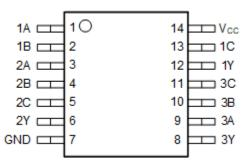
Figure 4-1. SN74LV27A D, NS, PW, DGV, or DB Package (Top View)
