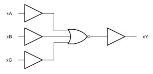
Figure 7-1. logic diagram, each gate (positive logic)
