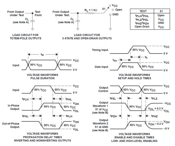
Figure 6-1. Load Circuit and Voltage Waveforms
