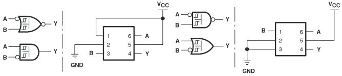
Figure 3. 2-Input NOR Gate With One Inverted Input 2-Input AND Gate With One Inverted Input
