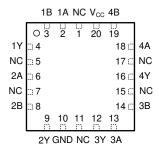
Figure 4-3. SN54LVC86A FK Package, 14-Pin LCCC (Top View)
