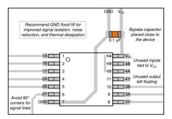
Figure 8-3. Example Layout for the SN74LVC86A
