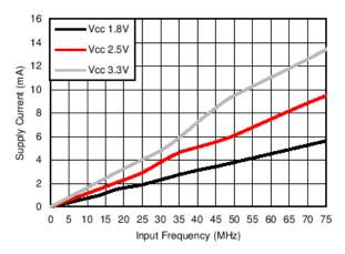
Figure 8-2. Supply Current vs. Input Frequency
